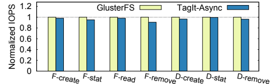
Figure 8: Metadata indexing overhead of TagIt for a large deployment. F- and D- denote the file and directory operations, respectively.
