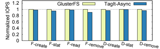
Figure 8: Metadata indexing overhead of TagIt for a large deployment. F- and D- denote the file and directory operations, respectively.
