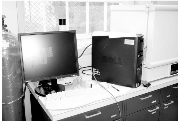
Figure 2. Experimental setup for thermal model validation. The box to the right of the workstation is the oven, with integrated drive electronics (IDE) cables coming out the door.
